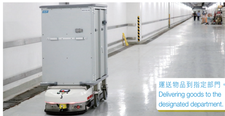
自動導航運輸車收到訊號，出發接載儲物箱。 An AGV heads out to pick up its storage cabinet.
