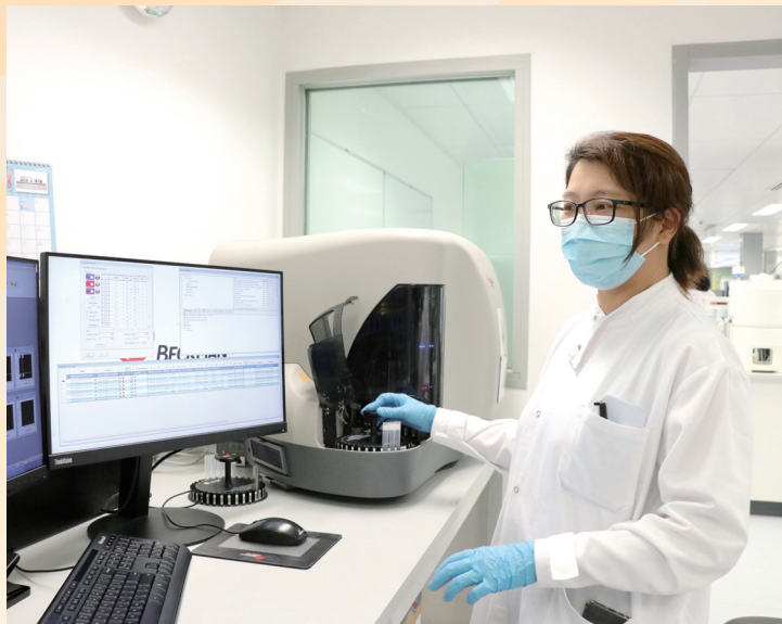
醫務化驗師運用流式細胞儀確認急性白血病類型和監察微量的殘餘癌細胞。 Using a flow cytometer to classify the type of acute leukaemia and monitor minimal residual disease.
